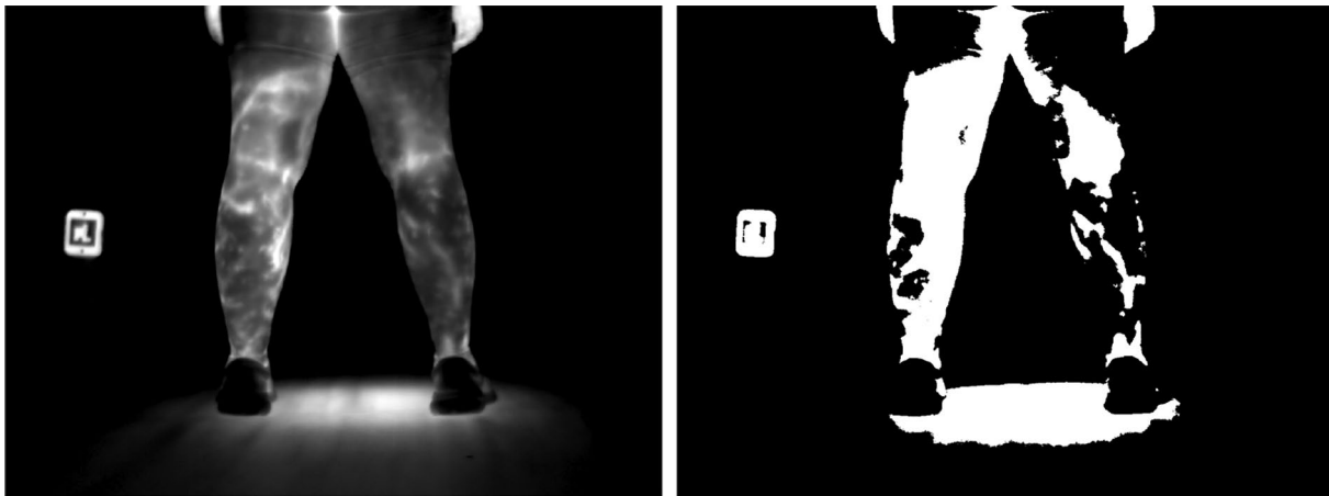
Fig. 6 Thresholding a thermogram results in an unclosed mask when applied to an exhausted subject. Left: thermogram; right: threshold with Otsu's algorithm.
