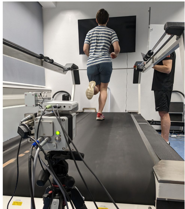
Fig. 7 Experimental setup with stereo camera setup in the foreground and a runner on a treadmill (left) and the operator of the treadmill (right) in the background. The upper camera is the Microsoft Azure Kinect, and the lower camera is the JENOPTIK VarioCam HD head.
