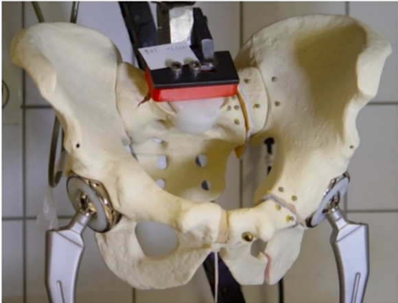
Fig. 3. Test setup with the bone model set on two fixed bipolar hip prostheses and connected to the lever arm of the servo-pneumatic test machine via end-plate of S1.
