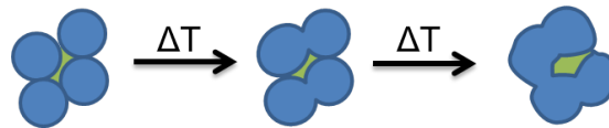
Figure 5.10.: Schematic illustration of the decrease in surface area (darker blue) and increase in pore size (green) upon heat treatment of the m\text{Ta}_2\text{O}_5 nanoparticles.
