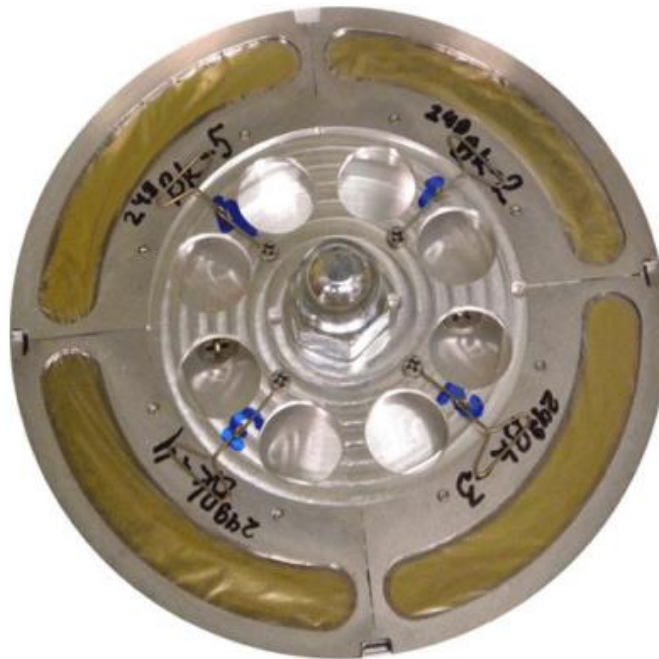
Figure 1.6: ^{249}\text{Bk} deposited with the molecular plating technique. The wheel is made of four target segments prepared individually [38].
