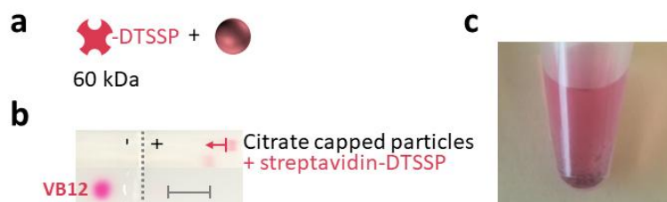
Figure IV-16. Particle modification with tetrameric streptavidin. (a) Sketch of the attachment procedure of streptavidin (tetramer) via DTSSP to a gold particle. (b) Gel electrophoresis image of citrate-capped particles and the same batch incubated with DTSSP-activated streptavidin. Scalebar: 1 cm. (c) Photograph of a dark residue in a streptavidin particle sample.
