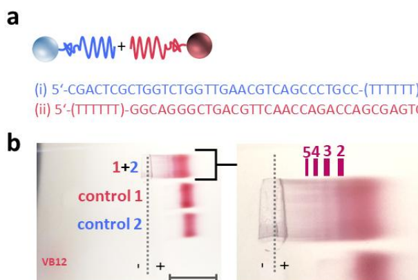
Figure IV-20. Hetero-type assembly, without Hsp90. (a) Sketch of the DNA-modified particles. The particles are pre-passivated with a methoxy-PEG and maleimide-PEG (2000 g/mol, 3000 g/mol). Thiol-capped DNA strands are attached via maleimide chemistry. In this example, the DNA is fixed at 10% via maleimide anchors. i-ii show the DNA sequences. 40 (b) Gel electrophoresis image of DNA particles (control 1 and control 2 are color coded according to sequences in i-ii), as well as the mixed sample. Closeup of the mixed sample (right) shows multiple bands beside the monomer band. Scalebar: 1 cm.
