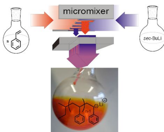
Figure 4.14: Schematic layout of anionic styrene polymerization in a microstructured reaction set-up in continuous flow.
