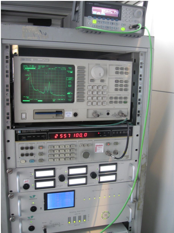
Figure 3.8: Overview of the main room temperature electronics and data acquisition devices used in SpecTrap. From top to bottom: Agilent 33250A - frequency generator HP 3589A - spectrum/network analyser HP 3336A - synthesized function generator Cryo Bias - power supply and room temperature amplification for cryo-electronics HV-500-8 - precision voltage supply QUAD 1-10 - rotating wall drive Not shown are DS345 function generators, HV power supplies and switches. The timing for switching the trap electrodes is realized with two DG535 digital delay generators, which are also not visible on the photo.
