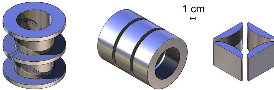
Figure 4.10: Drawing of a deflector, einzel lens and a multipole, respectively left to right, true to scale as used in the SpecTrap beamline.
