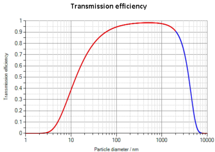
Figure S3.3. Transmission efficiency for the SP2 inlet system (from ambient to SP2 inlet), calculated using the Particle Loss Calculator in August 2022.
