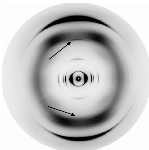
Figure 3.28. Scattering of microfocus synchrotron radiation for HBC-PhC 12 (performed by Dr. Mari Cruz García Gutiérrez at Grenoble, France). The arrows indicate the reflections.
