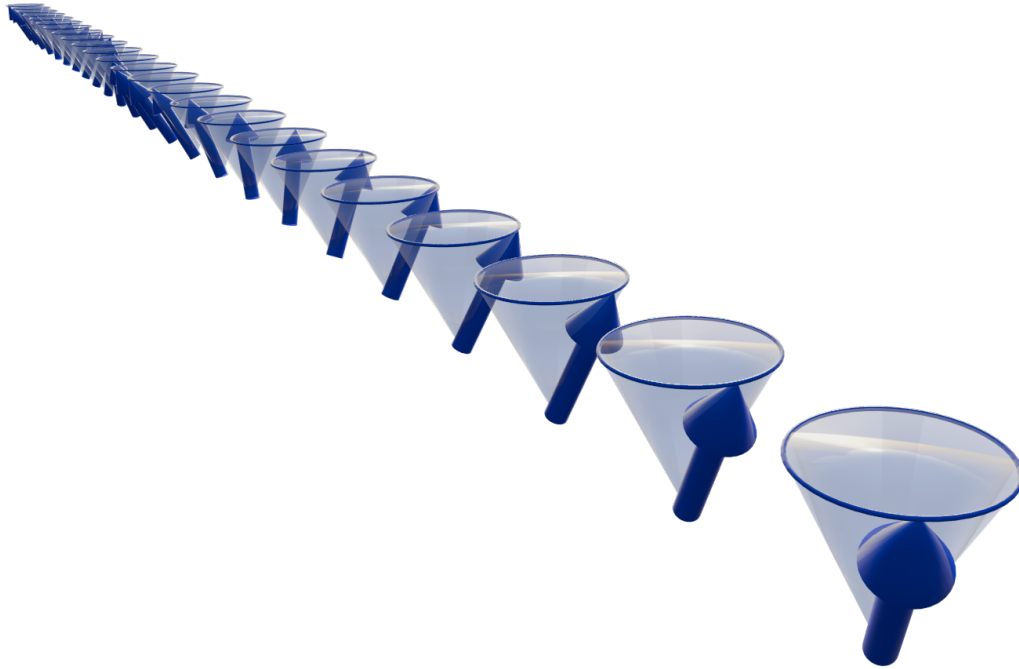
Figure 2.6: Spin wave. The spins perform a collective precession with a constant phase shift between neighboring spins
