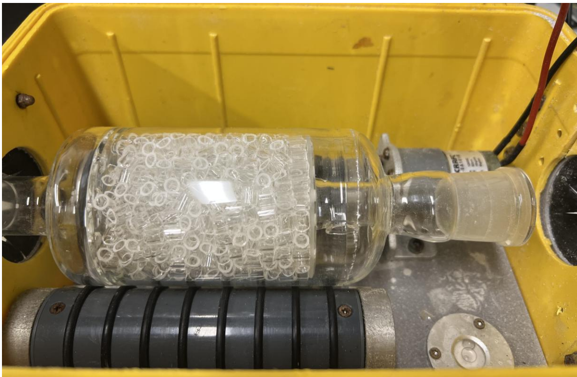
Figure 2: Rotating Raschig tube system consisting of a glass vessel filled with Raschig rings, mounted on two motor-driven rollers to induce rotation and continuous rewetting of the packing; the gas pump is not shown.
