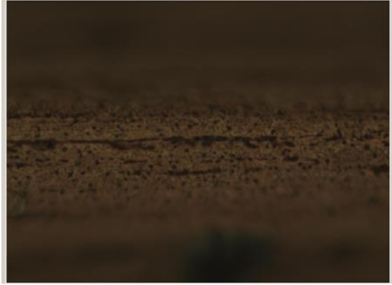
Figure 56: Optical microscopy picture (20x magnification) of a copper wire surface, coated with hexadodecyl-HBC after pyrolysis. The diffuse areas at the top and the bottom appear due to the convex surface.
