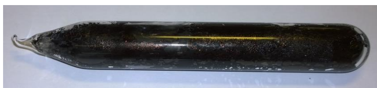
Figure 58: Picture of a quartz ampoule after pyrolysis, revealing carbonized material in its inside.
