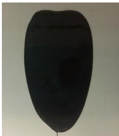
Figure 80: Example of a laminate of 42 with conductive carbon C65 and Kynar® binder in the ratio 60/30/10.
