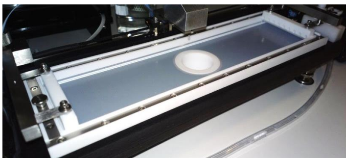
Figure 15: Picture of the liquid-liquid Langmuir trough, used for the assembly of 13 , 10 , and CB[8] at the toluene-water interface.
