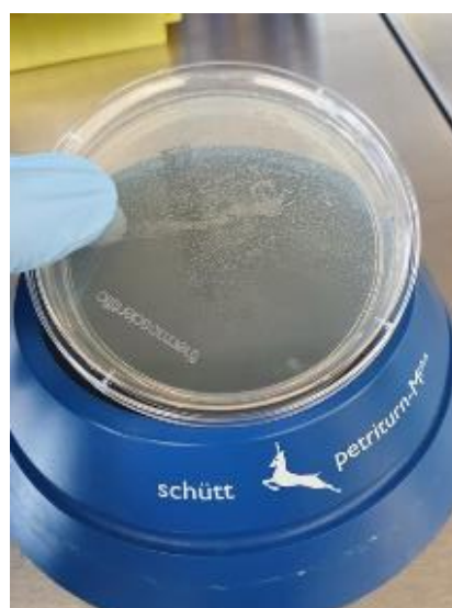
Figure 32: Dilution series of polymer N on MHA. Dilution of 1:1000 showing no CFU'S indicating antibacterial properties
