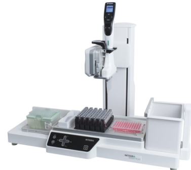
Figure 2 - INTEGRA Assist Plus pipetting robot
