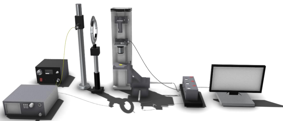
Figure 2.1 Illustration of the setup of 3D Photon Upconversion Direct Lithography (PUDL) process.
