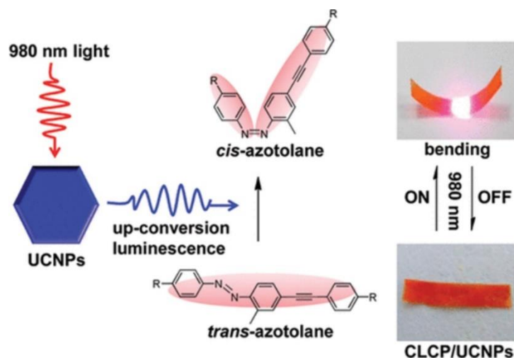
Figure 1.15 Schematic illustration of the UCNP-incorporated azotolane-containing liquid-crystal polymer film. Bending of the film was induced by NIR light at 980 nm. The upconversion luminescence of the UCNPs leads to trans – cis isomerization of the azotolane units and an alignment change of the mesogens. The bent film completely returned to the initial flat state after NIR light was turned off. Reproduced by permission of ref. 80. Copyright 2011, American Chemical Society.
