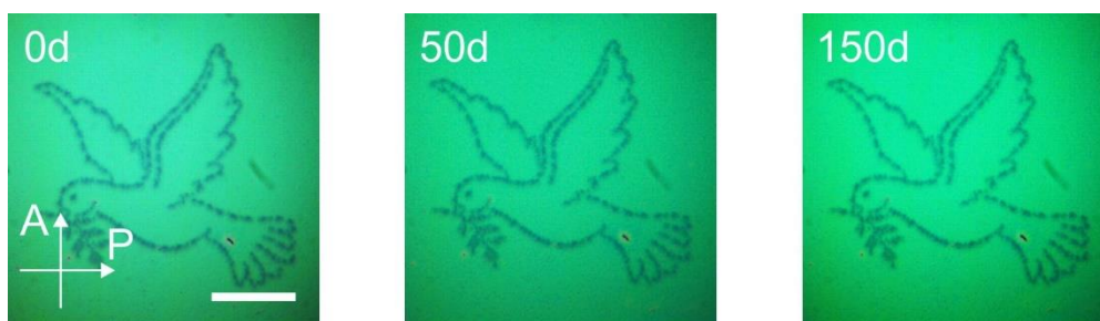
Figure 4.15 POM images of a peace dove pattern on PAzo/UCNP@PAzo film fabricated by PUDL process. The pattern can be store for more than 150 days in an office with natural light at room temperature.
