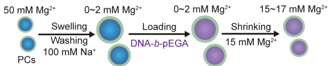
Figure S3.4. Schematic Loading Process. The PCs were washed with 100 mM Na + TE buffer to open the pores of the shell for better encapsulation of i *- b -pEGA. Subsequently, the concentration of Mg 2+ was adjusted to 15 mM to stabilize the PCs.
