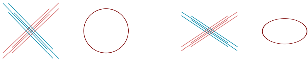
(a) Fiber bundles crossing at an angle of 90^\circ and the resulting DTI ODF.
