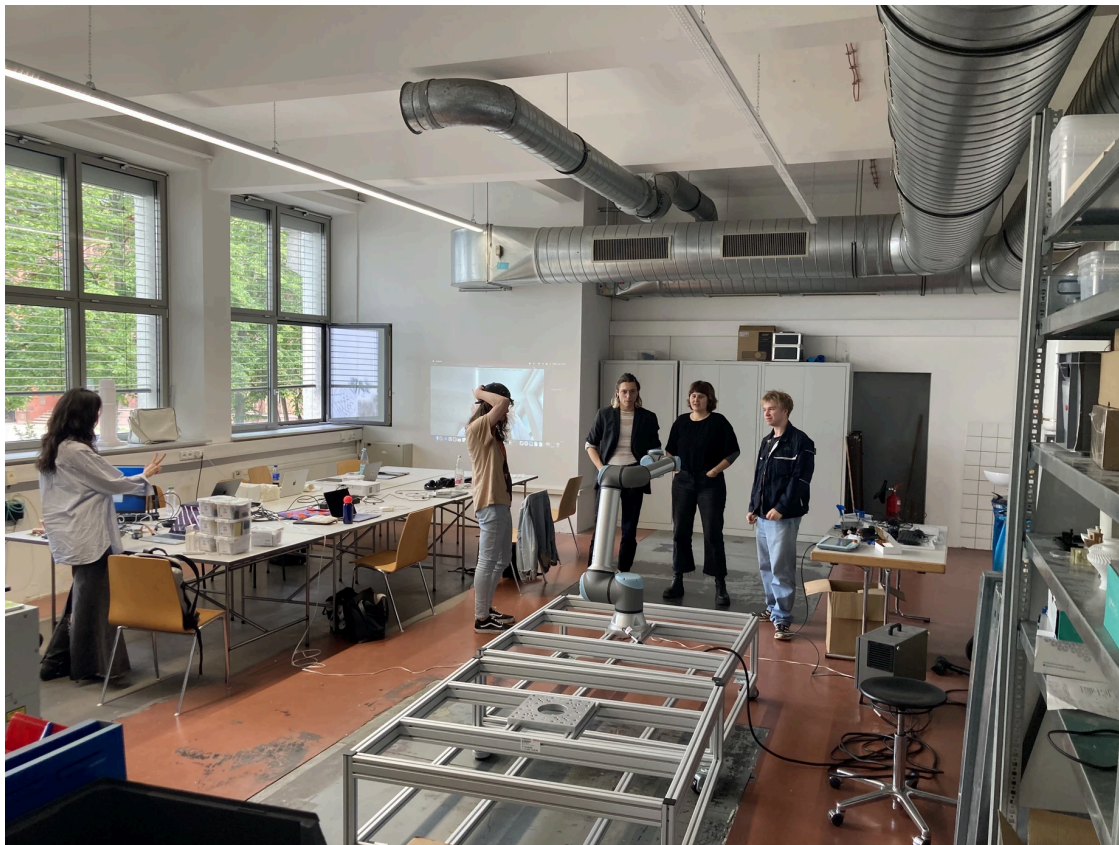
Figure 1: Students testing a custom hand pose model on a UR10e robotic arm, with each gesture triggering a predefined movement. © Ivan Iovine
