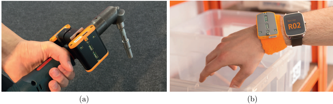
Figure 6.1: Example images from an official nexonar assembly scout advertising brochure 3 . These images show different cross-shaped HSRM-Tracking markers attached to a screwdriver (a) as well as a wristband (b). Here the markers are integrated in custom cases that include a battery and a USB power charging interface, designed by soft2tec GmbH.
