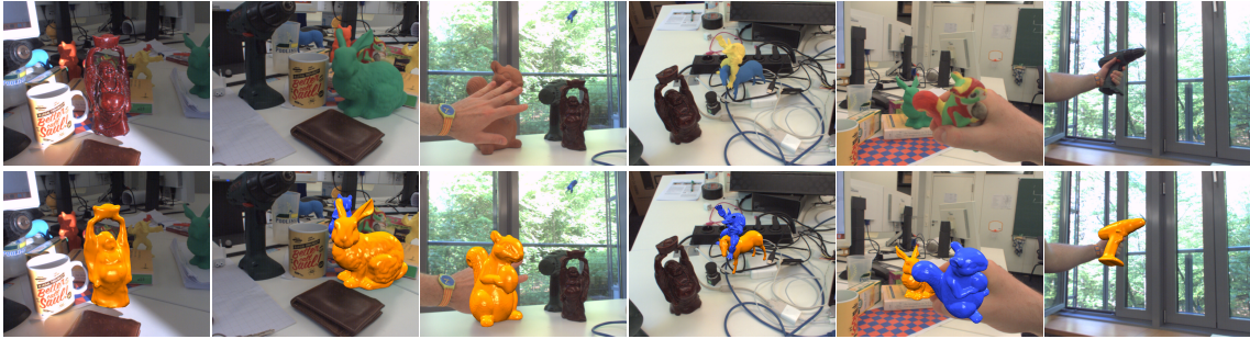
Figure 6.7: A few examples of the proposed passive method estimating the pose of a single or multiple complex objects under different challenging conditions. These include cluttered scenes/backgrounds, strong occlusions as well as direct sunlight. Top: The raw RGB input frames. Bottom: A mixed reality visualization of the tracking result where the input images are virtually augmented with renderings of the corresponding 3D models using the estimated poses. All results were obtained within \sim 16 ms per object.
