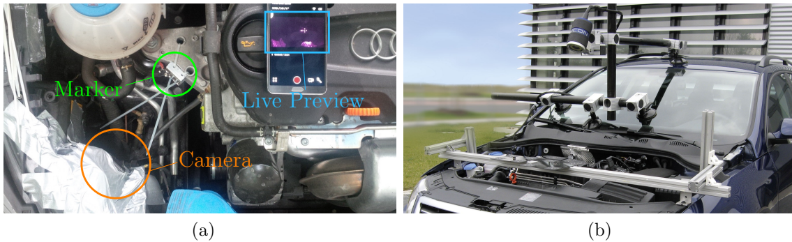
Figure 6.2: A photo of the experimental setup inside an engine compartment, using HSRM-Tracking for measuring the movement of a car’s engine block (a) in comparison to the EngineWatch system 6 of the AICON 3D Systems GmbH (b).
