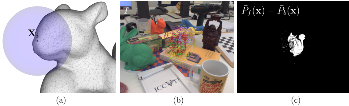
Figure 4.8: Object segmentation using tclc-histograms in the scene of Figure 4.6. Here, a tclc-histogram attached to a 3D vertex \mathbf{X}_i of the squirrel model is shown in a schematic 3D visualization (a). Due to this relationship each center \mathbf{x}_i of a local region \Omega_i can be identified in every frame. In this example this is illustrated by depicting the local regions as colored circles where the RGB value matches the relative object coordinates of the corresponding \mathbf{X}_i (b). Based on such tclc-histograms, the average pixel-wise posteriors \bar{P}_f(\mathbf{x}) and \bar{P}_b(\mathbf{x}) can be computed using (4.9), which provide an even higher quality object segmentation (see e.g. the bottom part of the squirrel) than the individual local posteriors in Figure 4.7 (c).
