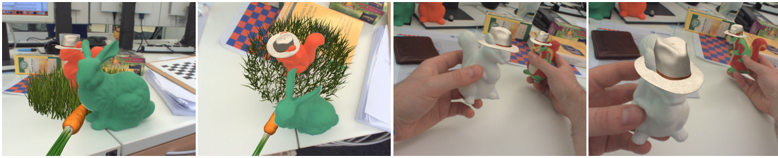
Figure 6.8: Mixed reality visualizations in two different complex scenes with two tracked objects each. Based on the pose estimates the real objects are augmented with virtual attachments (hats, a carrot and a patch of grass), in real-time. Here, despite large perspective changes and both modelled and unmodelled occlusions, the augmentations remain precisely in place.
