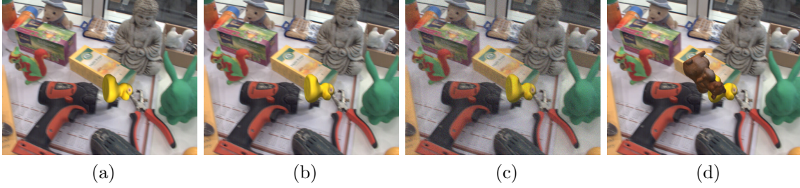
Figure 4.21: An example frame from the RBOT dataset with the duck model in the four different variants: the regular (a), the dynamic light (b), the noisy (c) and multi-object version (d) with occlusions. Visually comparing the regular with the dynamic light version clarifies the impact of the lighting aspect on the appearance of the object region.
