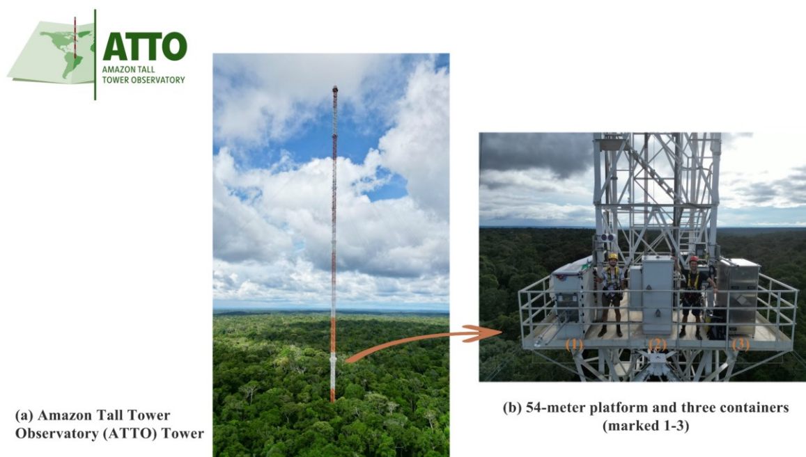
Figure 2.5: An overview of the ATTO measurement site. (a) The full view of the ATTO tower. (b) The 54-meter platform and three containers, from left to right, are equipped with the following instruments: (1) CIMS; (2) Nano-SMPS & PMS; (3) NAIS.
