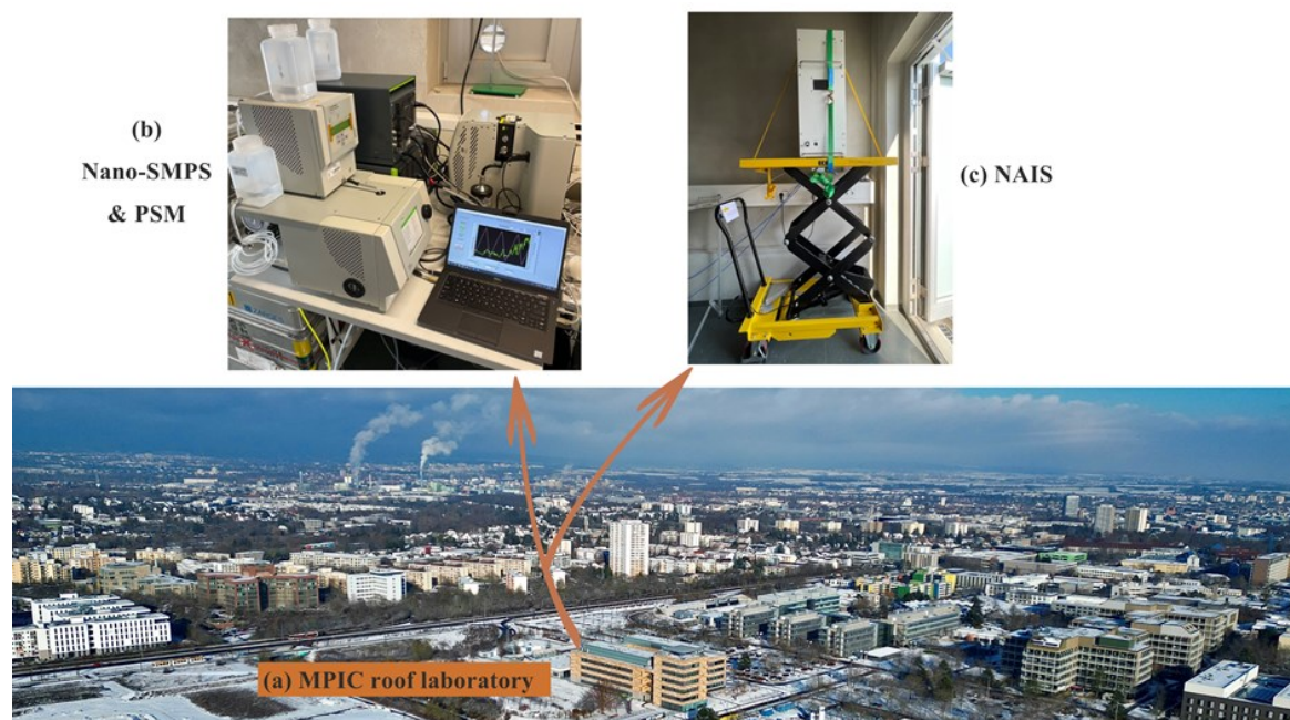
Figure 2.6: (a) The rooftop laboratory at the MPIC building and its surroundings. Photos of the instruments in operation in the laboratory (b) Nano-SMPS and PSM. (c) NAIS.
