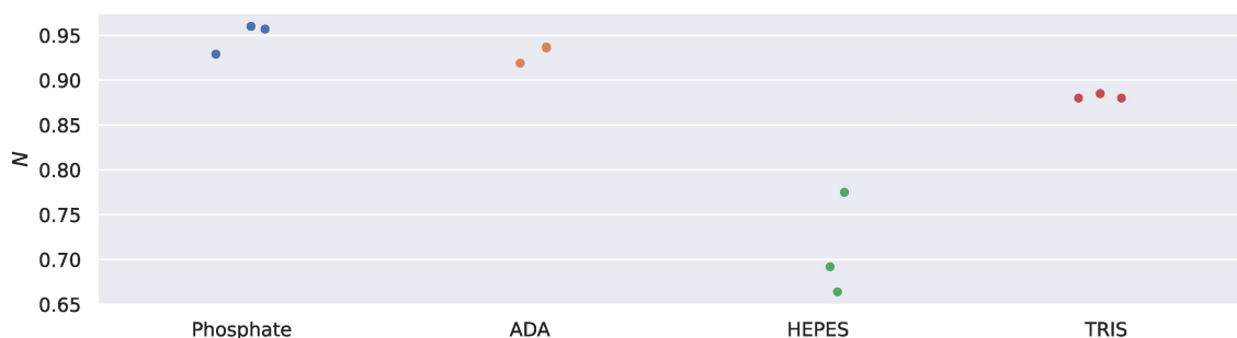
Figure 4. Overview of stoichiometry N of ITC measurements of the binding reaction between EP and pepA in different buffers of 100 mM concentration at a pH of 7.0.
