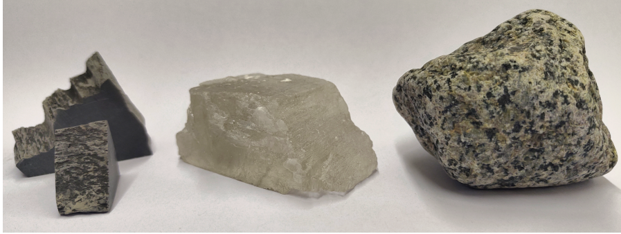
Figure 1.1: Examples for the three host rock systems considered suitable for long-term nuclear waste storage: argillaceous, salt and crystalline rock (left to right).
