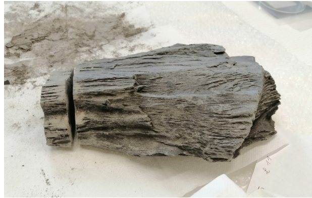
Figure 1.7: Piece of Opalinus Clay rock from the Mont Terri Underground Rock Laboratory used in publication II. From this piece small parts were sawed off and prepared for CNC milling to produce the diffusion cores.
