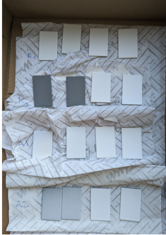
Figure 6.5: Primer and coating application tests on corten steel: Each row uses a different primer, indicated by R1, R2 (anti-rust primer) and A1, A2 (acrylic primer). In each row, the two left samples are only primed, while the two right samples are primed and coated with OPRC.
