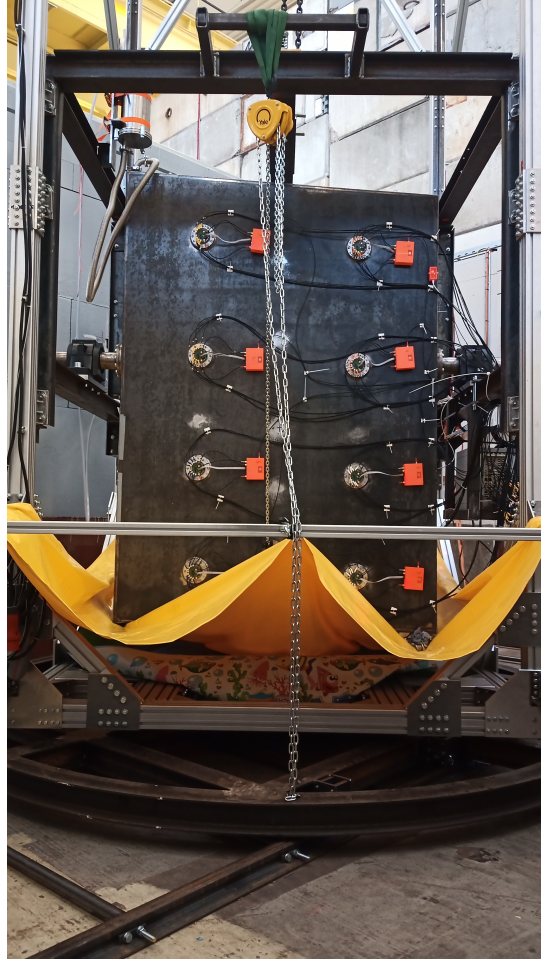
Figure 6.32: The 4-cell-prototype fully equipped with WOMs, SiPMs and readout electronics at the CERN test beam area
