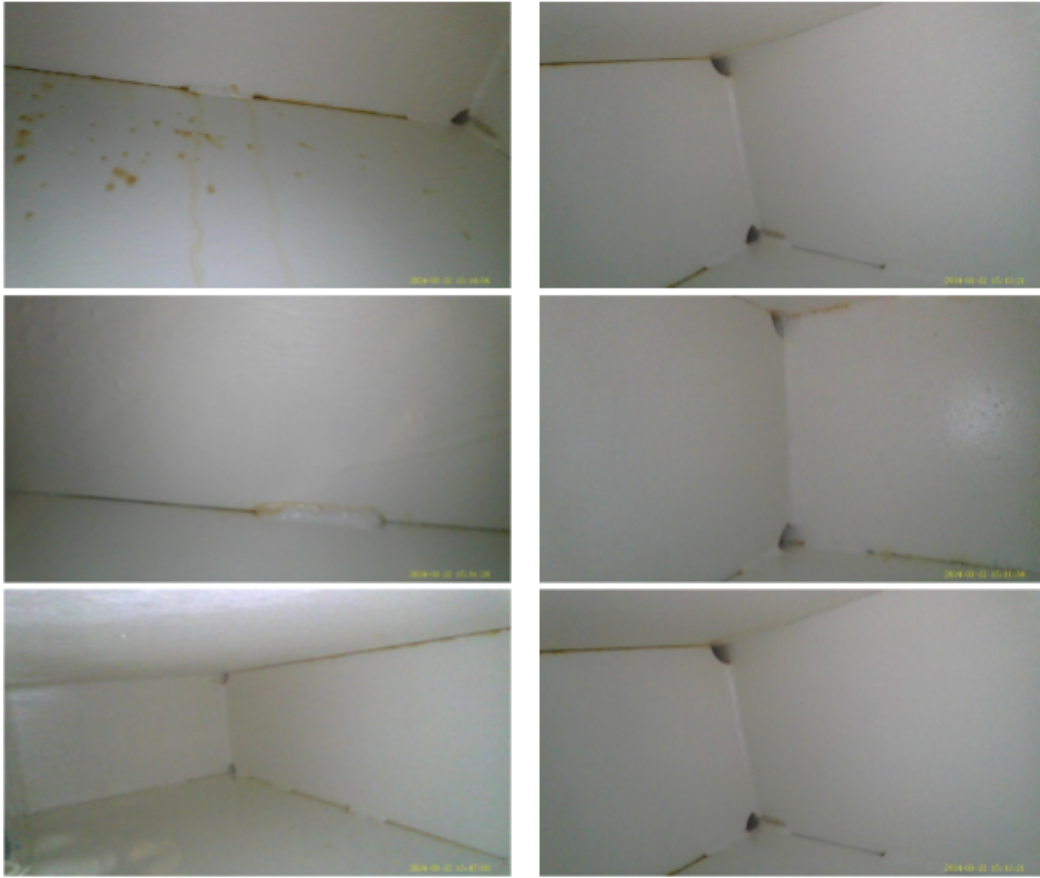
Figure 6.38: This figure presents additional endoscopic photographs of the 4-cell prototype, taken in March 2024. The focus here is on highlighting areas of the reflective coating that exhibit pronounced yellowing.
