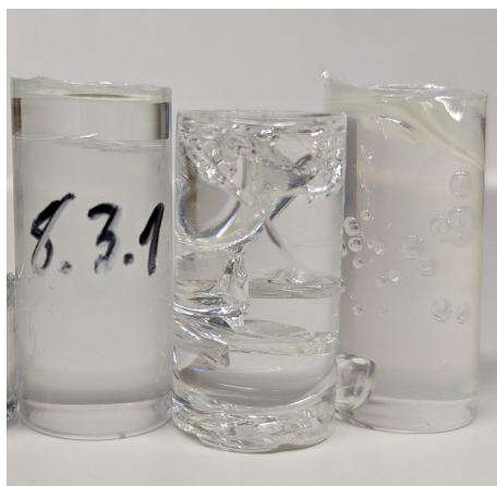
Figure 8.6: Plastic scintillator samples with different weight fractions of BPO added as an polymerization initiator (L-R: 0.5 wt.%, 1 wt.%, 0.1 wt.%).
