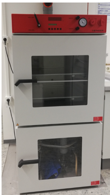
Figure 8.2: Vacuum oven used for the polymerization of plastic scintillators. The upper compartment houses the oven chamber, while the lower compartment contains the cold trap and the vacuum pump.
