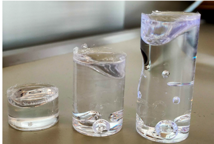
Figure 8.5: Three identically produced polystyrene samples show the dependency of bubble formation on the volume of the individual samples
