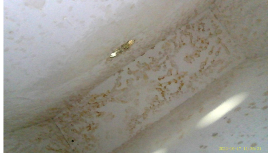
Figure 6.27: Final coating result of the top half of the 1-cell-prototype
