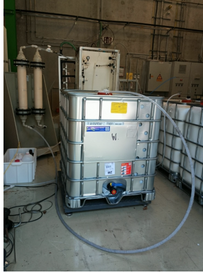
Figure 5.5: LAB purification setup at the Max Planck Institut für Kernphysik in Heidelberg for the purification of 1000l of LAB. Raw LAB is pumped from one IBC, through aluminum oxide columns into another IBC, where the purified LAB is collected. Two columns with 10 kg of Aluminum oxide each are sufficient to purify up to 350l of scintillator.
