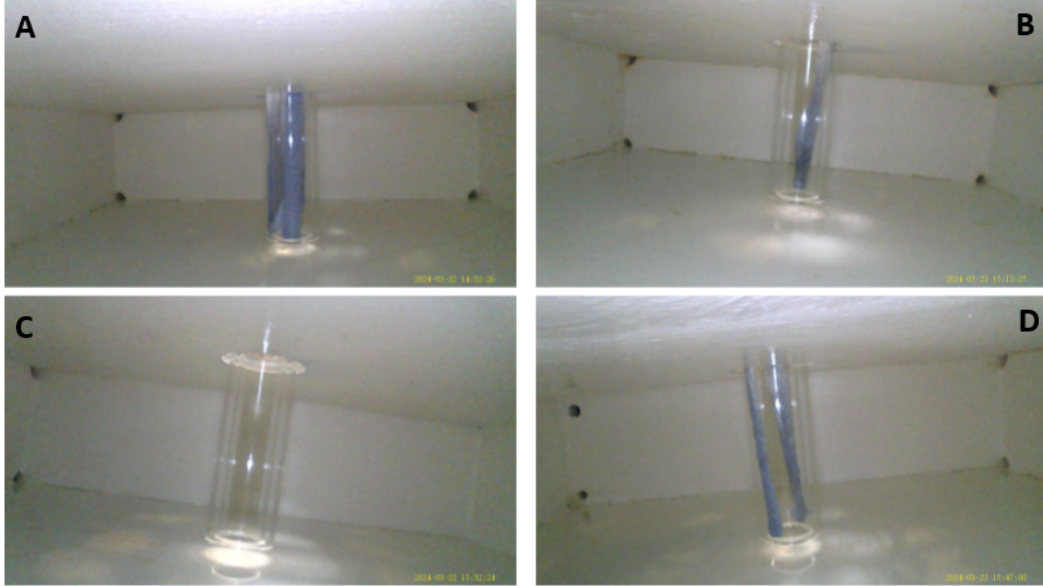
Figure 6.37: This figure presents endoscopic photographs of the inner walls of the 4-cell prototype, taken in March 2024. By this time, the reflective coating had been in contact with the liquid scintillator for four months. Each photograph corresponds to one of the individual cells, showing the condition of the reflective coating in that cell.
