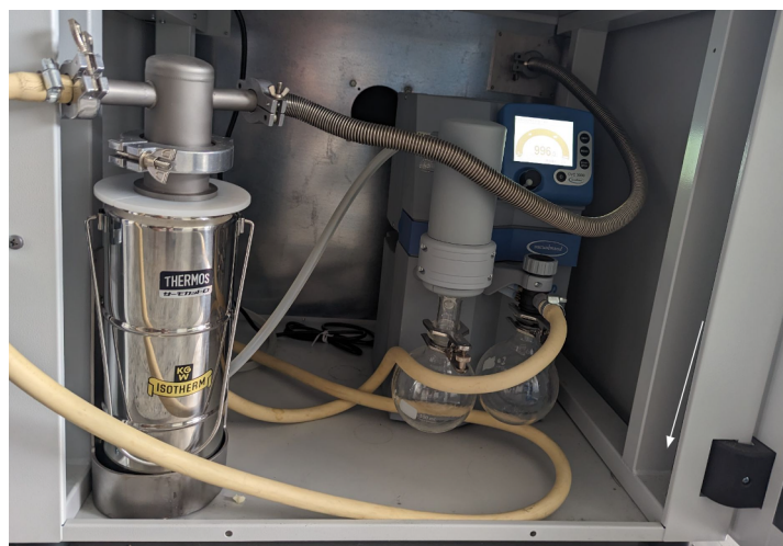
Figure 8.3: Cold trap (left) and vacuum pump (right) located in the lower, ventilated compartment of the polymerization setup.
