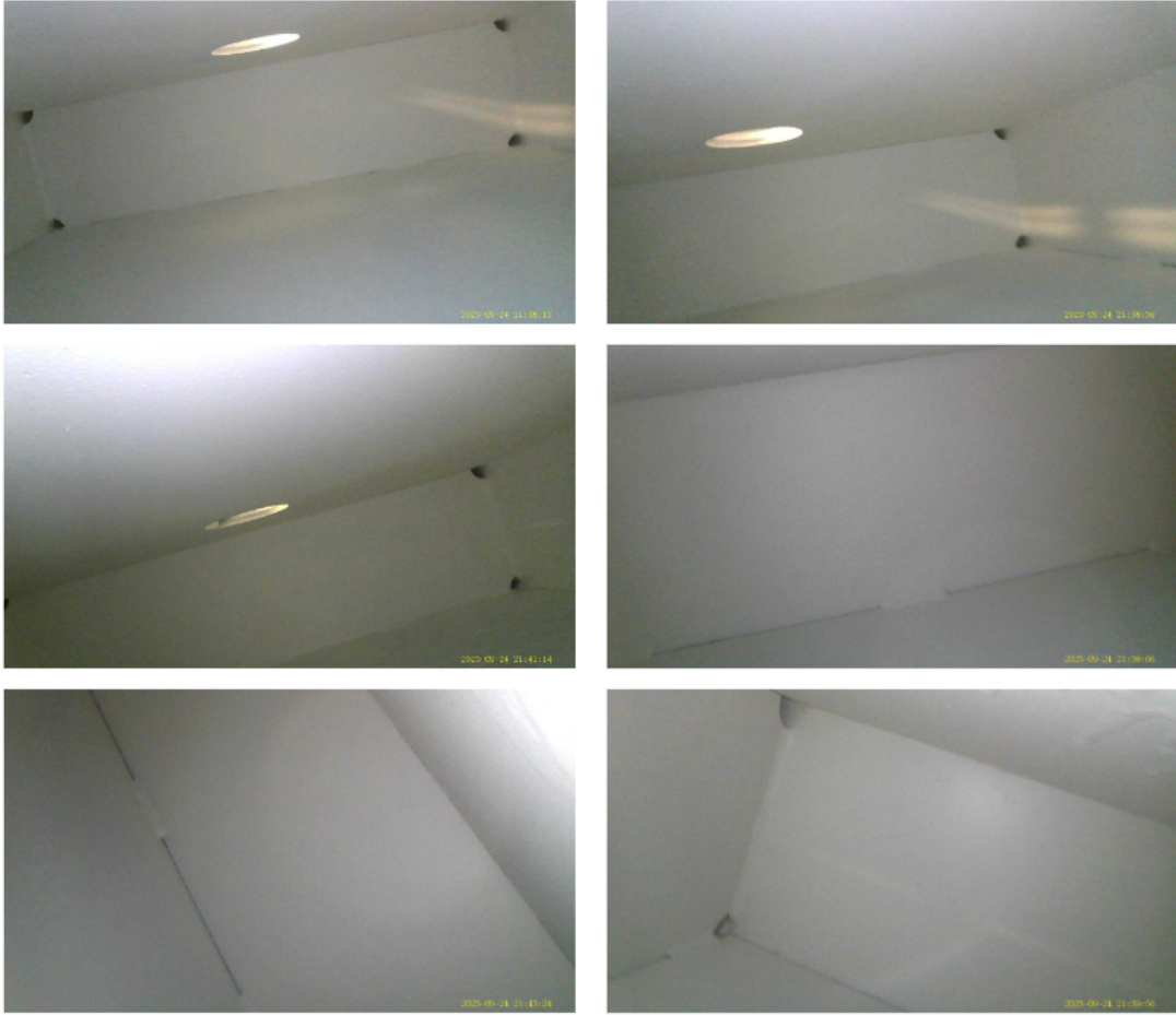
Figure 6.35: A selection of endoscopic photos taken of the inside of all cells of the 4-cell-prototype after completion of the coating process
