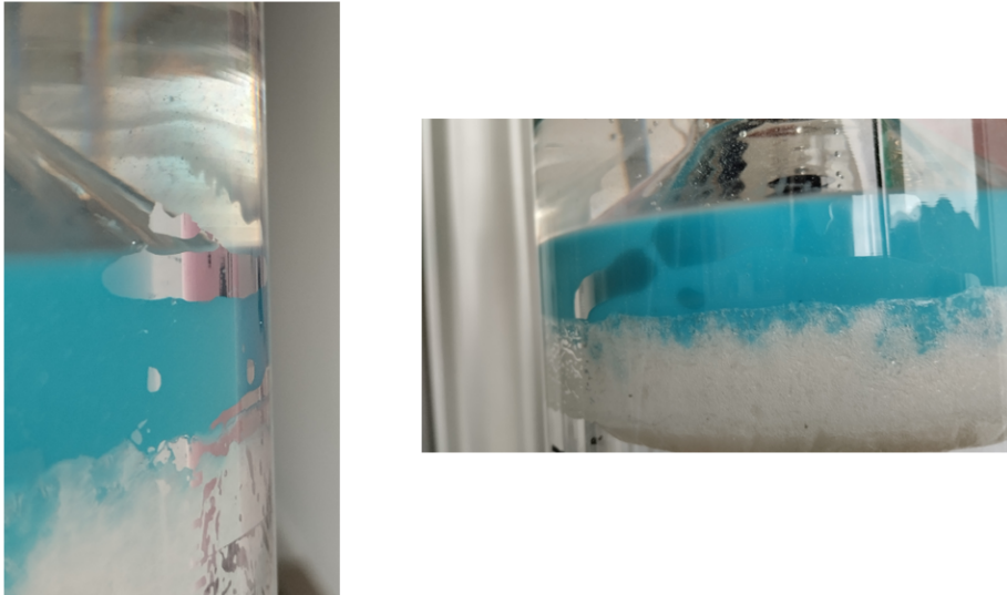
Fig. 9.11.: Blue silicon layer at top PMT during push-pull test at 0.3 bar pressure difference. We see air bubbles along the MoldStar silicon layer indicating movement of it due to the pressure difference. This effect is not seen on the ShinEtsu layer, which has a much better glass adhesion.
