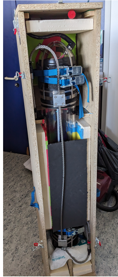
(b) Final box design used to ship the modules to the South Pole.
