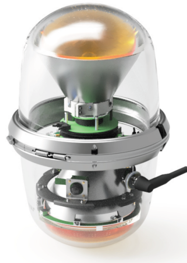
Fig. 3.6.: Design of the D-Egg [41]. It uses two large PMTs pointing up and downwards.
