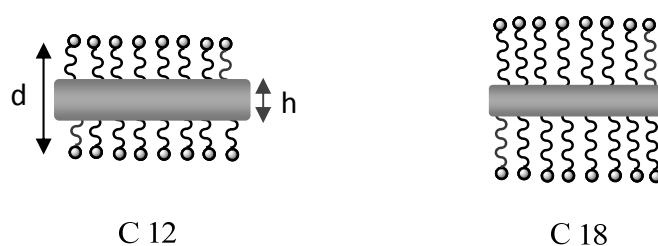
Figure 5.18 The interacting volume for 16- DSA incorporated in a C12 bilayer is higher than in a C18 bilayer. The interacting volume represents the effective volume for spin exchange and is determined by the bilayers width d (e.g. the surfactant chain length) and the flexibility of the doxyl- label hydrocarbon chain. In this picture the chains are fully extended, which will never be the case but illustrates the maximum height of the interacting volume. In a C12 bilayer, the flexible 16-DSA chain end can bend back and, hence, the nitroxide has more degrees of freedom which will also increase the possibility for spin exchange.
