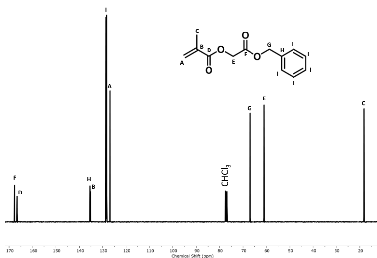
Figure S12: ^{13}\text{C} -NMR spectrum (101 MHz, \text{CDCl}_3 ) of benzyl protected glycolic acid modified methacrylic acid (MA-Gly-Bn).
