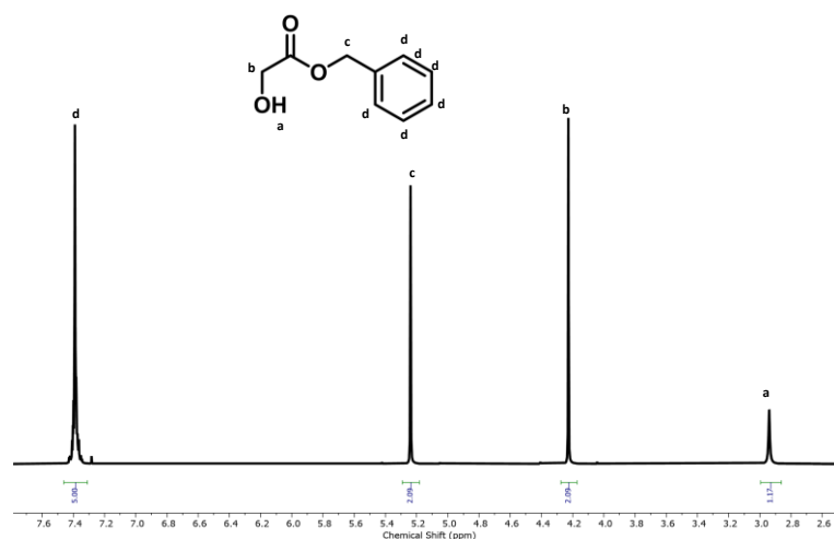
Figure S1: 1 H-NMR spectrum (400 MHz, CDCl 3 ) of benzyl protected glycolic acid (Gly-Bn).
