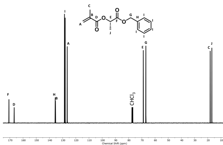
Figure S17: ^{13}\text{C} -NMR spectrum (101 MHz, \text{CDCl}_3 ) of benzyl protected L-lactic acid modified methacrylic acid (MA-Lac-Bn).
