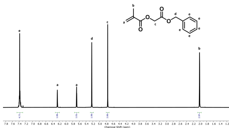
Figure S11: ^1\text{H} -NMR spectrum (400 MHz, \text{CDCl}_3 ) of benzyl protected glycolic acid modified methacrylic acid (MA-Gly-Bn).
