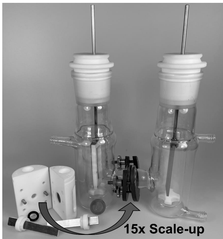
Figure S2: Comparison of the different cells used. Left: Teflon™ screening cell with 6 mL per half-cell equipped with SIGRAFLEX™ and stainless-steel electrodes, Nafion™ N324 membrane and EPDM-O-Ring. Right: jacketed glass cell with 90 mL per half-cell equipped with a Nafion™ N324 membrane, SIGRAFLEX™ and stainless-steel electrodes, Teflon™ plug and electrode holders.
