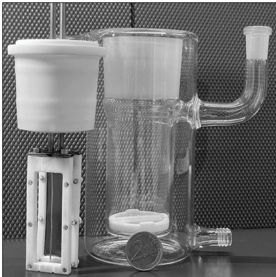
Figure S2: 100-mL quasi-divided glass cell with Sigraflex™ anode and stainless-steel wire cathode, electrode holders and stirring bar used for the scale-up experiment. Diameter of the coin 25.75 mm.
