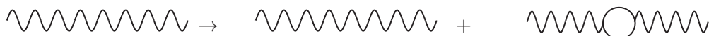
Figure 2.A.1: Vacuum polarization insertion in the photon propagator to first order in \alpha .
