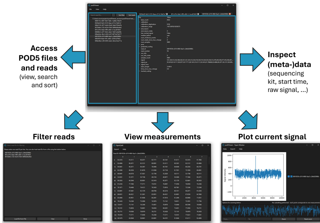
Figure 1. Overview of the pod5Viewer and its main features. Top: Main window containing the navigator (left) and data view panel (right). Bottom left: Read filtering to show only a specific subset of reads. Bottom center: Data viewing function showing individual measurements. Bottom right: Plotting function for visualizing the current signals for opened reads.
