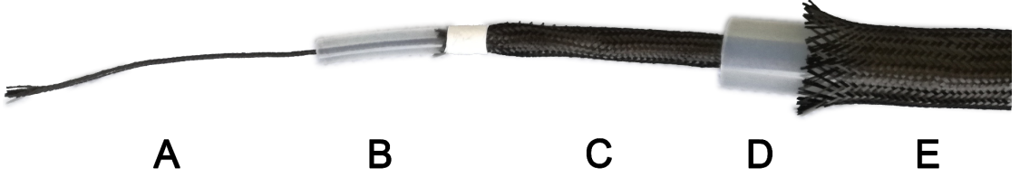
Figure 3.11.: Picture showing the composition of the HV cable. The conductors A , C & E are carbon mesh tubes, the insulators B & D are silicone tubes.
