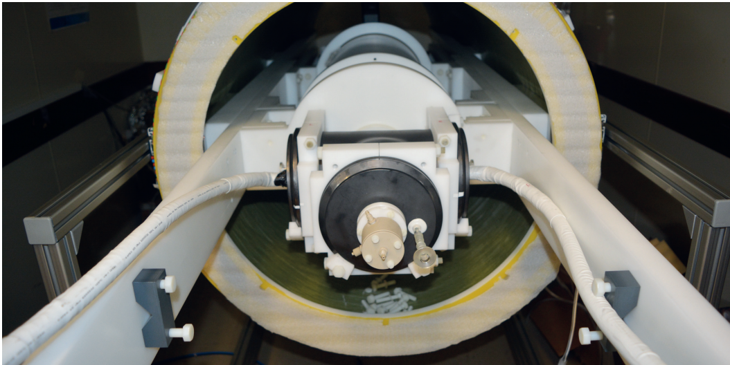
Figure 3.2.: Picture of the fully assembled EDM setup with view from the bottom of the setup. The rail system is attached to the GRP tube; the EDM casing (black) is mounted below the SQUID cryostat on the carriage. For the picture the carriage is partially moved out of the GRP tube.
