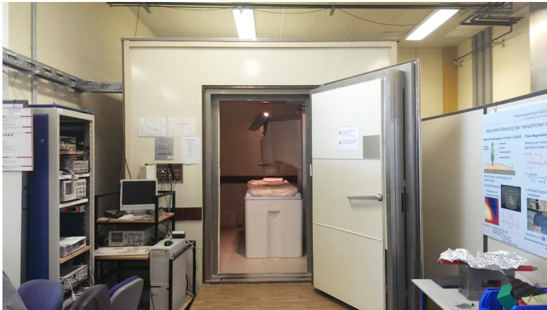
Figure 3.12.: Status of the MSR in Jülich at the beginning of the Xe-EDM initiative: inside of the room is an examination couch for a test person and a liquid nitrogen cooled SQUID system mounted on a gantry that was used for low field MCG measurements.
