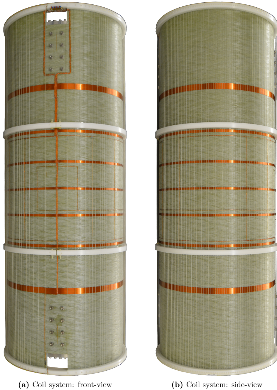
Figure 3.22.: Front- (a) and side-view (b) of the coil system mounted on the GRP cylinder. The thin vertical wires form the loops of the cos-coil. These bow-taut wires are hold in place by four well-aligned white rings made out of POM. Openings on top and bottom of the cylinder, clearly recognizable in the front-view picture (a) are used as a passage for the gas filling line, cables and other supply lines. Furthermore, the seven ring coil segments of the solenoid configuration, which are directly glued onto the GRP tube, are discernible. More difficult to recognize are the windings of the gradient coils. The wires forming a two-times fork-like shape in picture (a) are the supply-lines of the individual coils, twisted in pairs with opposite current directions to prevent interfering fields.
