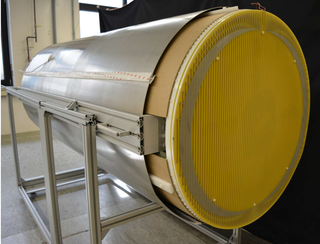
Figure 3.23.: A picture of the fully assembled magnetic field system: The mu-metal cylinder is surrounding the coil system which is protected by two half-shells of cardboard. The removable lids of the cos-coil are attached with plastic screws. An access on the side for the several connections and the gas filling is clearly visible, just below the lid in front. The setup with a height of \approx 210 cm is pivoted on a movable cart made out of aluminum that fits through the door of the MSR. If necessary for maintenance, the whole setup can be moved out of the MSR without disassembling. When moved and turned in its final position, the (magnetic) wheels of the cart can be exchanged by non-magnetic and vibration-damped legs.
