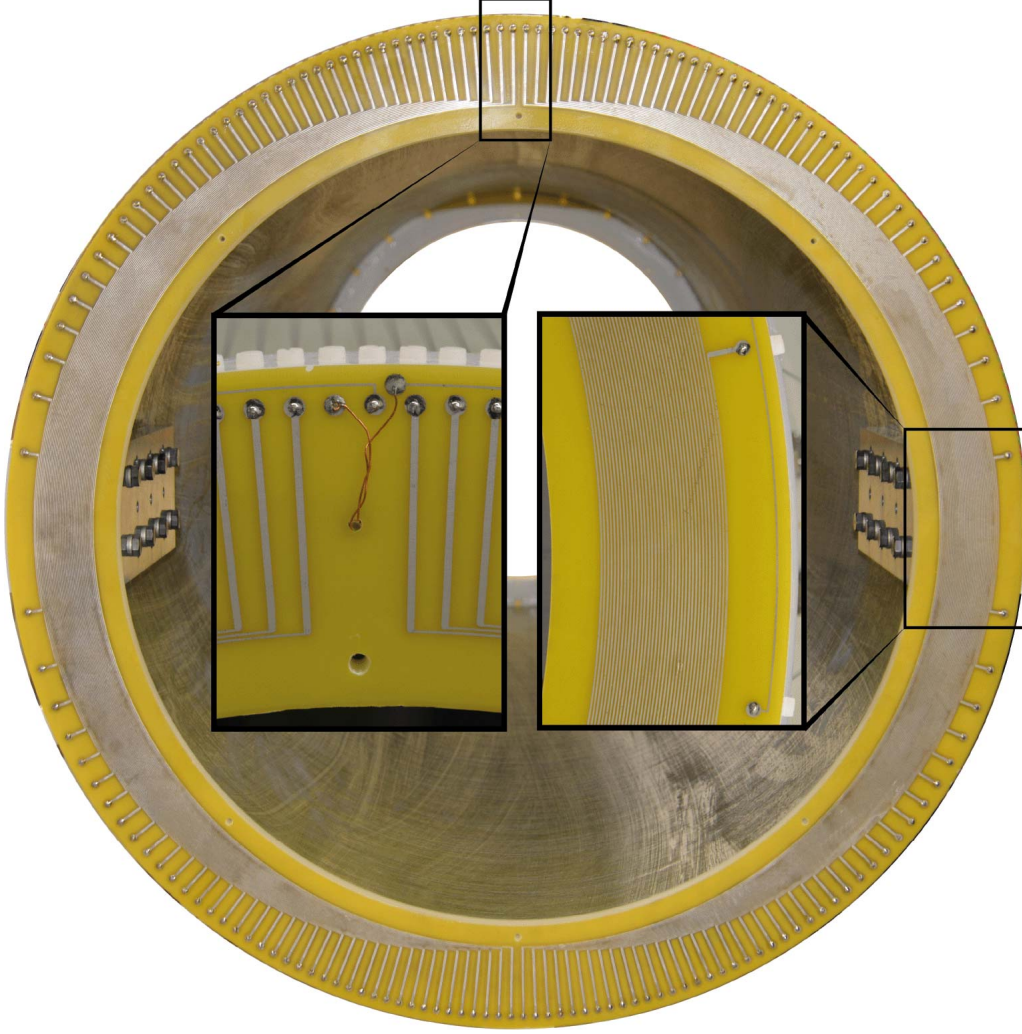
Figure 3.20.: Picture of a bypass ring of the cos-coil system. The wires are connected to loops by bypass lines, which are printed on a circuit board.
