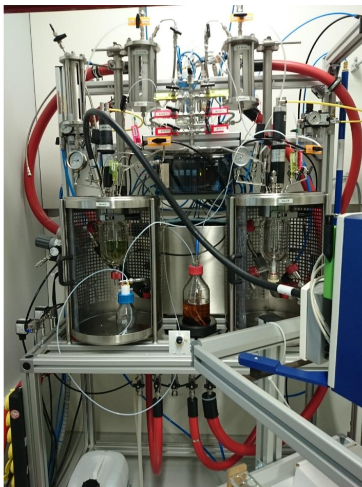
Figure S 1. Photograph of the reactor setup used for the safe addition of ethylene oxide to a preheated reaction mixture.
