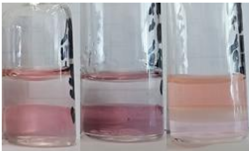
Figure S 18. Solutions of hbPEO_{0.34}\text{-}C18_{1.00} (0.01 wt%) saturated with dye (bottom layer) after agitation with aqueous solutions of sodium hydroxide with increasing concentration (from left to right: pH 11, pH 14 and concentrated aqueous NaOH) (top layer).
