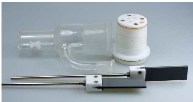
Figure S2: 25 mL beaker-type electrolysis cell; size of electrodes: 3 mm x 20 mm x 60 mm.
