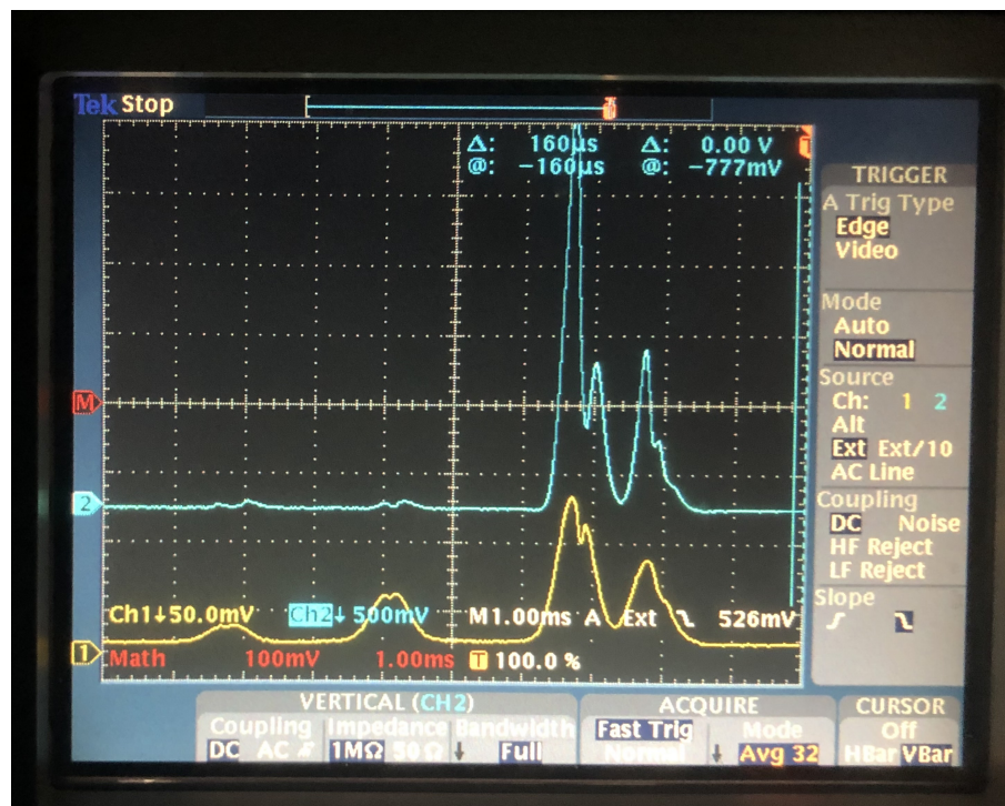
FIGURE 7.12: Backward beam experiment in Ashtarak. Backward-direction detection at zero field in Ashtarak. The blue line in the oscilloscope is the signal in the backward direction and the yellow line is the fluorescence.
