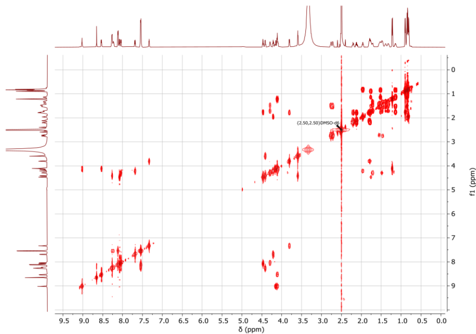
Figure 5: ^1\text{H} NMR and ^1\text{H} , ^1\text{H} COSY NMR spectra (700 MHz, DMSO- d_6 , 298 K) of compound 2
