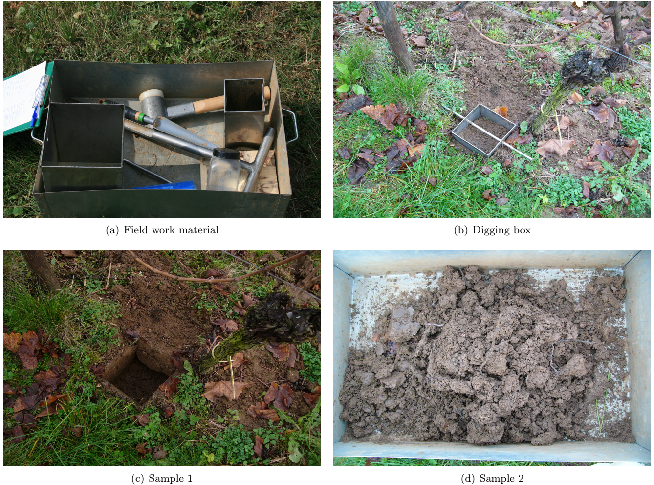
Figure 5: A: Field work material. Shown are small and big digging boxes, drill for soil sampling, plastic tubes filled with water for root transportation. B: Digging box in soil. C: Soil sample for root extraction. D: Root extraction from soil.
