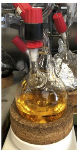
Figure S2. Polymerization reactor with orange color due to polystyryllithium (PSLi) chain ends before coupling reaction.
