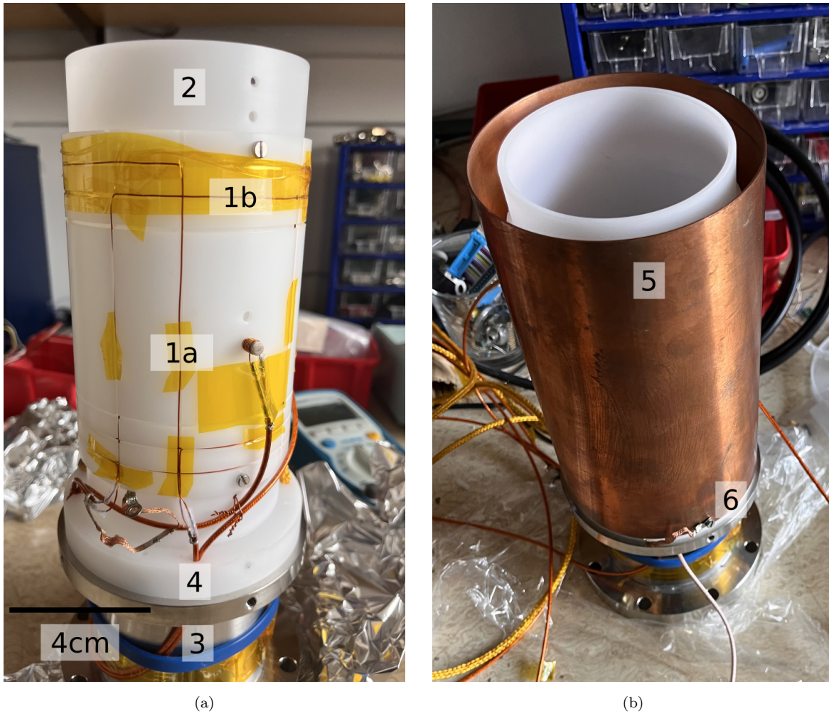
FIGURE 4.5: (a) Picture of SF1 without the rf shield. The saddle coils C1 (1b) and C2 (1a) are wound on the POM cylinder (2). For mounting in the translation stage, the POM cylinder is connected to a short stainless steel piece (3). The saddle coils are connected to coaxial cables which are fed through the POM cylinder (4). (b) Picture of SF1 with the copper rf shield (5) surrounding the POM cylinder. The copper shield is connected to the ground potential of C1 through a screw connection (6).
