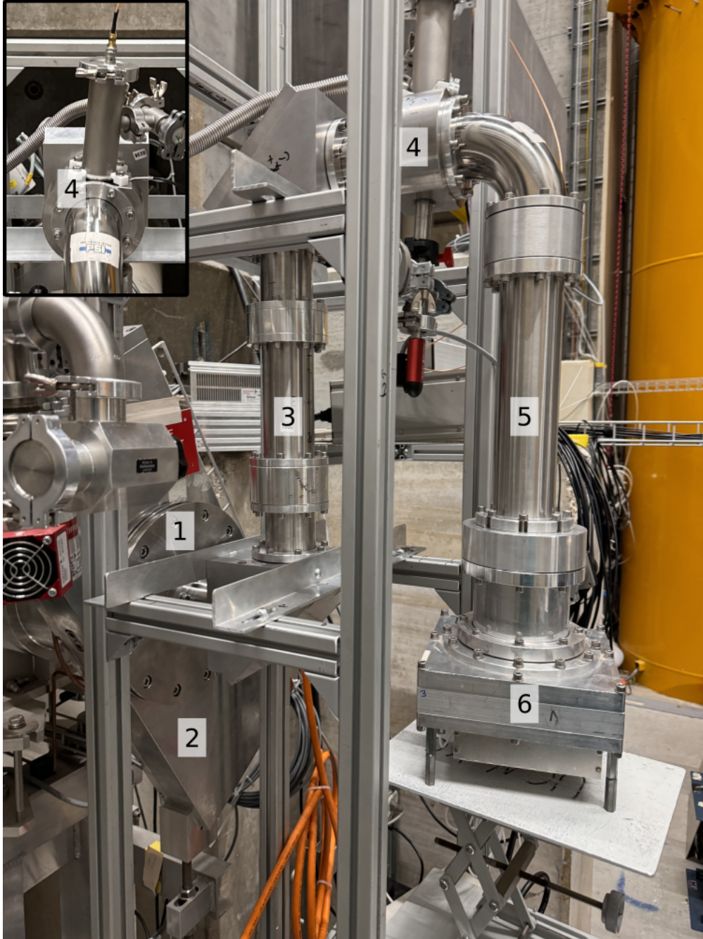
FIGURE 5.30: Setup for test measurements of the monitor-detector version 2 at beamport West-1 at PSI: UCNs enter the beamline through the beamport (1). The beamport can be closed using the vacuum shutter (2). Behind the shutter, the beamline (3) rises to a height of 59 cm above the center of the beamport, where the monitor detector is positioned (4). A close-up of the detector flange is shown in the top left corner. Inside the detector flange, a pinhole allows only a fraction of the UCNs to reach the detection surface. Behind the monitor detector, the beamline (5) goes down to the beamport height again, where the CASCADE detector (6) detects the majority of the UCNs.
