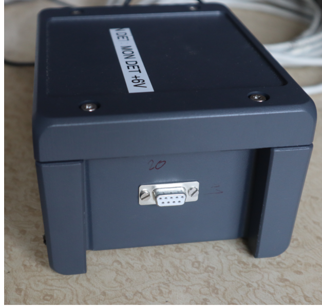
FIGURE 5.11: Housing of the monitor-detector version 1 electronics. Both PCBs and the micro-controller are inside the housing. The SiPMs are connected to the front using a sub-D type connector and a shielded multi-wire cable. 6 V supply voltage is connected at the back using banana plugs. The connection from the PC is done via a USB-cable. Ports at the side of the housing can be used to measure the SiPM supply voltage directly.
