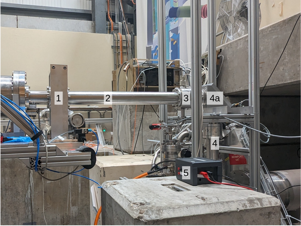
FIGURE 6.1: Picture of the monitor detector version 1 in operation with \tau SPECT at PSI. The entrance shutter of the experiment (1) is connected to the detector flange (3) by a horizontal 66 cm long piece of beamline (2). The detector flange is mounted to the top of the vertical beamline section (4). The bottom of the vertical beamline section is connected to the beamport. ^{58}\text{Ni:Mo} (85:15)-coated plates mounted at a 45^\circ angle are used to direct the UCNs through the 90^\circ angles on the top (4a) and bottom (covered by the concrete block) of the vertical beamline. The monitor-electronics version 1 (5) can be seen in the foreground. When the experiment cryostat is moved to another height, the length of the vertical section is adjusted.
