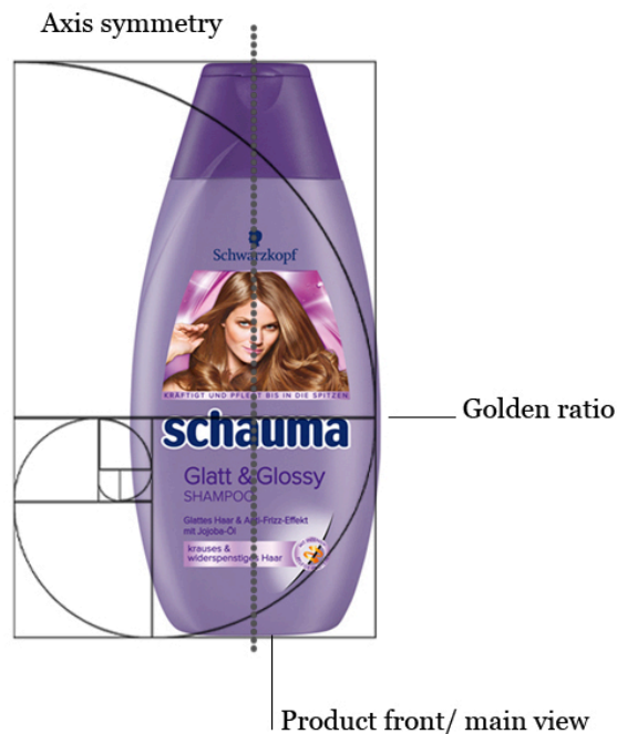
Image 38 SCHAUMA Shampoo Bottle: Axis symmetry, golden ratio and product front/ main view
