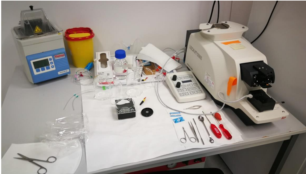
Figure 12. Picture of the Leica vibratome setup and the instruments in our lab arranged for the next brain slice preparation.
