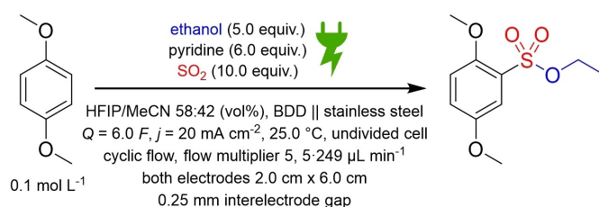
Scheme 2. Reaction conditions for the stability test. The yield, conversion, and selectivity (= yield / conversion) for each of the 10 runs was analyzed using quantitative ^1\text{H} NMR spectroscopy with 1,3,5-trimethoxybenzene as internal standard.
