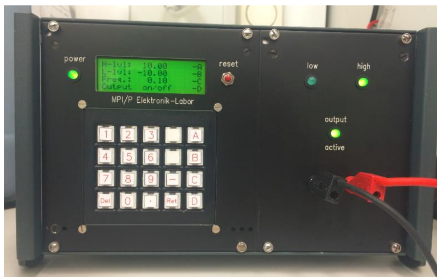
Figure S1 Home-made low-frequency generator as power supply for graphite exfoliation. The output voltage can be tuned from -12 V to 12 V, frequency from 0.01 Hz to 20 Hz.
