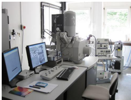
Figure 3.2. SEM column scheme (left panel) and the picture of FEI NovaNano 630 SEM used by the author.
