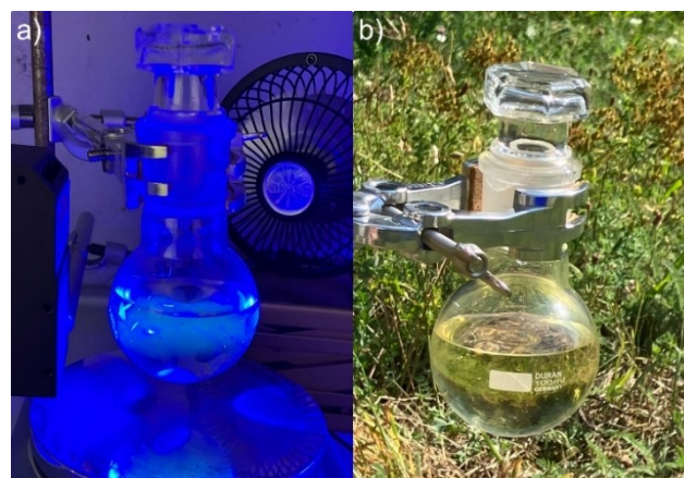
Figure 4. a) Photograph of the laboratory scale irradiation setup using a 100 mL round-bottom flask and a 460 nm UHP-LED. Intensity lowered to 5% to reduce overexposure on the photograph. b) Photograph of the irradiation setup using a 100 mL round-bottom flask and sunlight.
