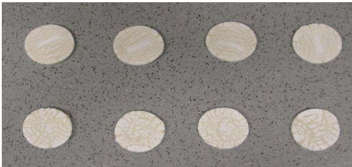
Figure 4-5. Chewing gums of uniform surface area after pressed with “Home Depot” method Upper row representing Nicotinell 2 mg mint and below is the Nicorette 2mg freshmint. Average surface area exposed to the drug release medium is approx. 11.39 cm 2 .
