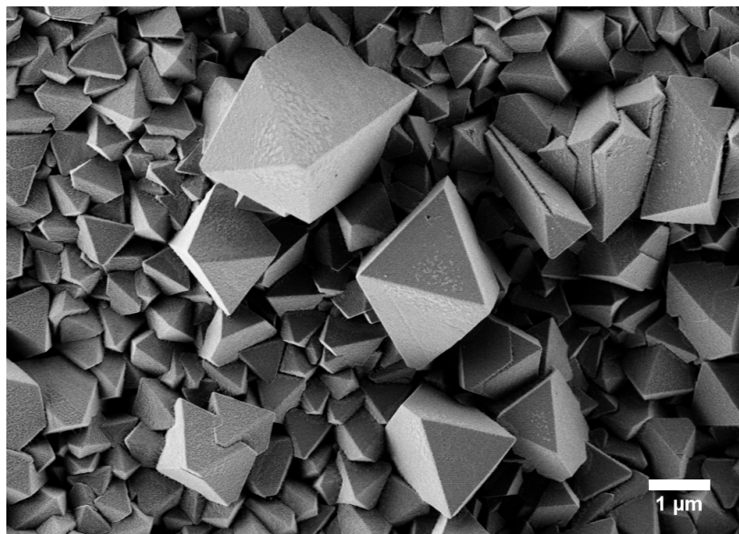
Figure 2.7 Scanning electron micrograph of a CuBTC coating on a copper substrate. Scale bar: 1 \mu\text{m} .
