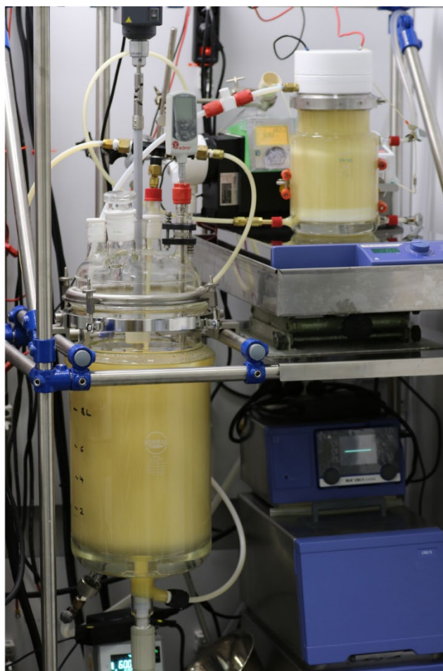
Figure 8. Reaction setup of the upscaled e-CSTR. Left: tempered reservoir with agitator. Below: thermostat. Above: eductor piece in black. Right: reactor with electrode stack. Behind: membrane pump. In the background, an Erlenmeyer flask with fresh substrate and a peristaltic pump for substrate feeding are installed. The overall reaction volume is up to 13 L. The yellow color of the reaction mixture in a later reaction stage can be visually perceived.
