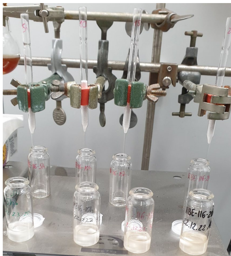
Figure S4. Workup of four samples, in the front row. The mini columns in the back contain \text{MgSO}_4 as drying agent.
