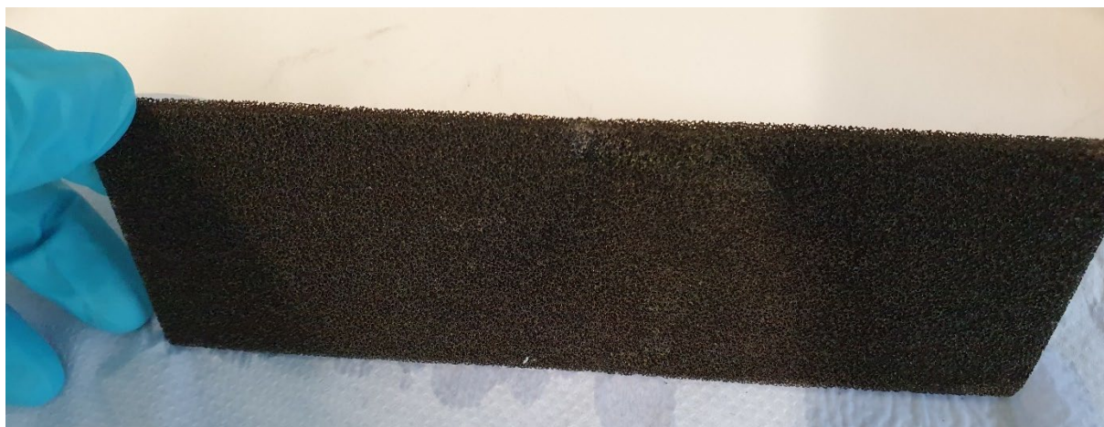
Figure 6. Activated RCM-Ni4753.05 nickel foam with a thickness of 5 mm and an average pore size of 0.4 mm. 67 The black nickel oxide hydroxide has covered the surface homogeneously.
