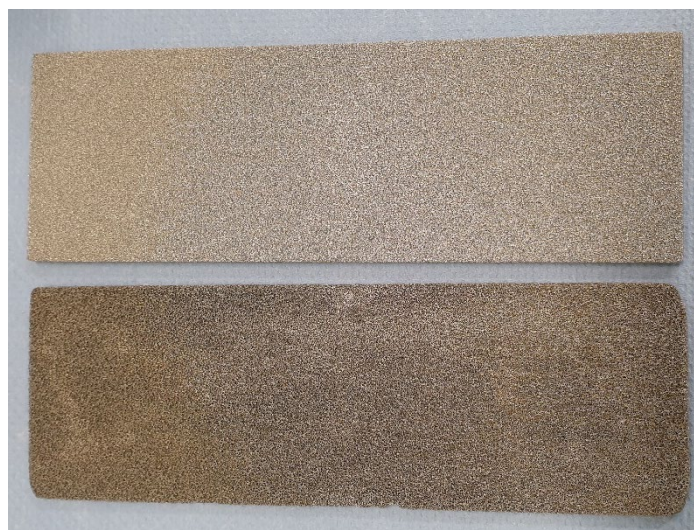
Figure 7. Top: New RCM-Ni4753.05 nickel foam. Bottom: RCM-Ni4753.05 nickel foam after ca. 50 reuses. Dimensions of the nickel foam: 60x180x5 mm 3 .
