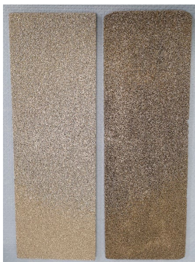
Figure S8. Image of pristine nickel foam electrode (left) and one after several uses and cleaning procedures (right).
