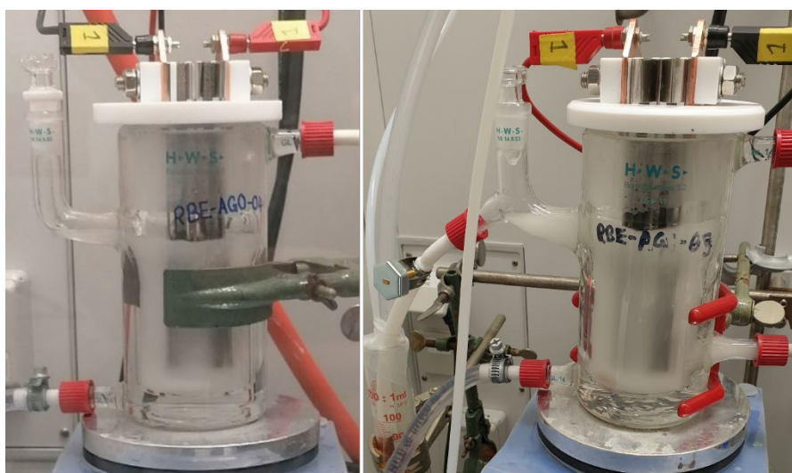
Figure 5. The transition from the batch-type cell for the first DoE (left) to the semi-flow mode electrolysis cell for the second DoE screening (right).
