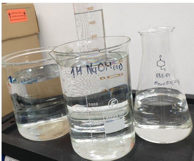
Figure S5. Exemplary image of the electrolyte for a V_{\text{tot}} = 13 L reaction. 11.6 L caustic soda (1 M) and 1.4 L of 1 ' are inserted into the reaction setup.
