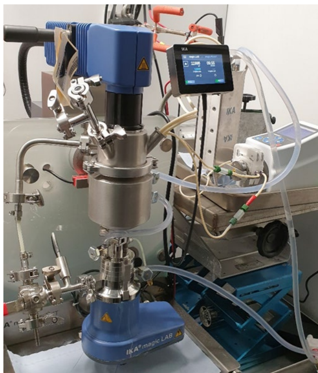
Figure 6. Setup of the reaction system: IKA magic LAB and magic PLANT mixing system (left half), moreover functioning as a reservoir; peristaltic pump (right); and the IKA ESF 6x18 flow electrolyzer (behind the pump).
