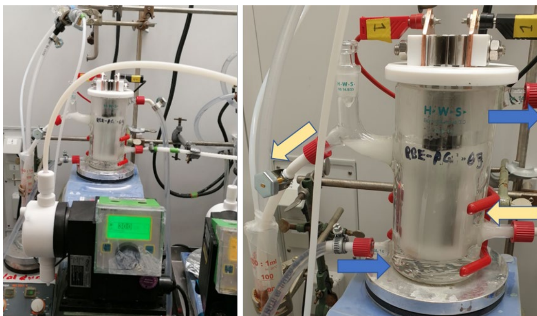
Figure S2. Setup with semi-batch electrolysis cell, eductor, membrane pump and reservoir. Light yellow arrows indicate the flow direction of the reaction medium, while blue arrows show the direction of the heating circuit.
