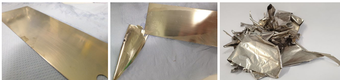
Figure S7. Left: During several consecutive activation runs in the cause of the screening, nickel was deposited on the stainless steel cathode. Middle: The nickel layer could be stripped of with a tweezer after the electrode was immersed in 4.5 M \text{H}_2\text{SO}_{4(\text{aq})} for a few seconds. Right: About 1.5 g of nickel were deposited in the course of these activation reactions.
