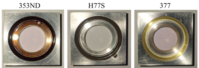
FIG. 4. Photographs of the aluminum viewports, including a window after curing of the stated adhesives. 377 shows an increased leakage of adhesive into the viewport, indicated by the ring formation around the clear aperture.
