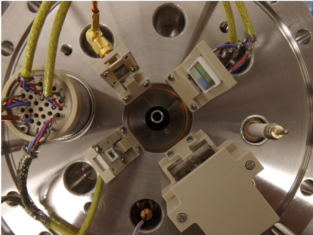
Figure B.26.: Sensor configuration in the test setup during the measurement runs. In the upper right corner is the Hamamatsu model S10942, then (clockwise) the 1" PMT R8520 from Hamamatsu, the Hamamatsu model S13370 MPPC and in the upper left the sample from KETEK. As can be seen the signal from the KETEK is connected via a SMA connector, the cables for the Hamamatsu MPPCs are soldered to pins, where the MPPCs are plugged in. In the center the drain pipe for the xenon is visible. Also the fibers can be seen which lead to a small, hollow PTFE cylinder placed in front of every sensor, to provide a diffuse illumination for calibration.
