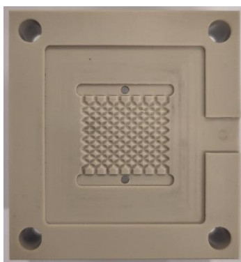
Figure S3: Photograph of the CO 2 compartment in the electrolysis reactor with an integrated flow-field for mechanical GDE support (cf. Figure S1).
