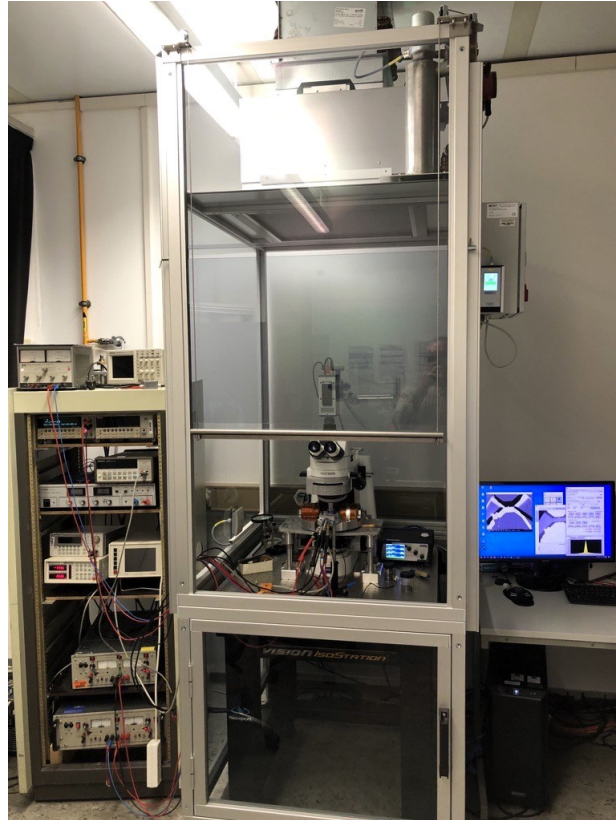
FIGURE 3.14: Full microscope setup with device rack on the left and PC on the right. The microscope is placed on top of a vibration reduction table and inside the laminar flow box. Temperature and flow control on the right upper side of the flow box.
