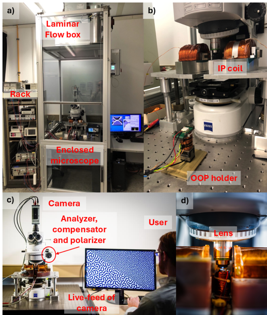
FIGURE 3.9: a) Schematic overview of the Kerr microscope setup. The system is based on a modified Zeiss AX10 wide-field microscope, enclosed within a laminar flow box and mounted on a vibration-isolated optical table. Peripheral components such as power supplies, temperature controllers, and auxiliary instruments are housed in the adjacent equipment rack. b) Close-up view of the optical table in front of the microscope. The OOP coil and its holder are positioned in front of the black x-y-stage, which is mounted on the microscope's focus stage. The IP coil is placed on a separate support, mechanically decoupled from the focus stage. c) Microscope equipped with a camera system mounted above the optical path. The camera delivers a live image feed - typically displayed via differential imaging (see Section 3.3.2) - to the control PC and user. Magnetic contrast is optimized by appropriate adjustment of the analyzer, compensator, and polarizer. d) Detailed view between the IP coil arms. The OOP coil holder, mounted on the focus stage, is located directly beneath the objective lens. Pictures c) and d) were taken professionally for AG Kläui.
