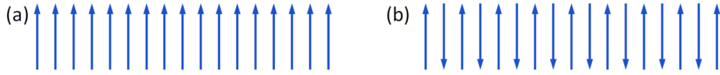
FIGURE 2.1: Schematically aligned spins from a) ferromagnetic and b) an antiferromagnetic structure. Taken from [22].
